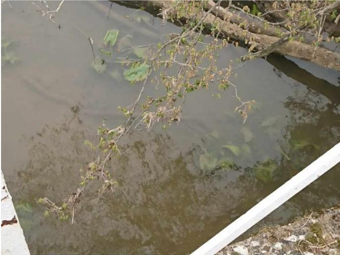
Presence of macrophytes in one the locations of field study. If the loggers are located close to it, the observed water temperature will be very lower than the other parts of the stream.
